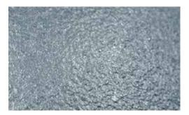
Ti6Al4V with porous titanium coating, magnified
